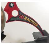
\*approximately 5 ½" down from the center of the wheel and 7 1/8" from the front edge of the wheel, with Wolverine set-up, per David Ellsworth's instructions<sup>1</sup>. It is about 1/16" farther away than a 50 degree Raptor jig setting.
