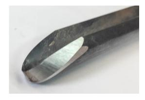
First of all, it is important to note that the Ellsworth gouge is either ½" (\$101.75) or 5/8" (\$121.75), and has a parabolic flute shape (left), not "U" (right) or "V" shaped. You can't get the same grind on a gouge
