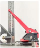
Now to find the settings for your adjustable jig, insert the gouge in the jig (backwards), clamp the open flute to a flat surface, and adjust the leg to get the same 148 mm "A" measurement as the Ellsworth jig. This sets the angle of the adjustable leg, one of the 3 variables.
