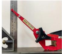
Clamp the front of the adjusted jig to a flat surface, and measure the distance of the pivot point to the front of the jig. This gives a 1-2 measurement of 139 mm for the Vari-Grind, and 148 mm for the Tru-Grind.
