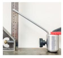
Next measure the distance from the pivot point to the front of the Ellsworth jig, parallel to the gouge (1-2) by clamping the front of the jig to a flat surface. This is also 148 mm.
