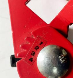
I number the positions from the top, and call this setting #5 for Oneway Vari-Grind, and #4+ for the Woodcut Tru-Grind. I also mark or scribe a line on the jig so I can return to the same setting repeatedly.
