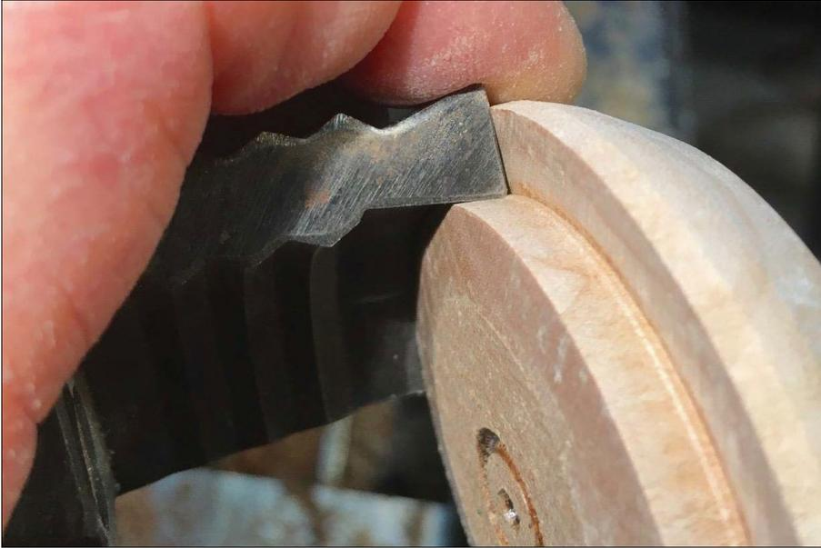
Have you ever made a tenon for a scroll chuck only to reverse your bowl and discover it doesn't turn true? If you understand what shape and dimensions are required for a tenon to fit the jaws of your chuck most securely, and then make the tenon accurately, your bowl will turn truer and reduce the time required to retrue it.
