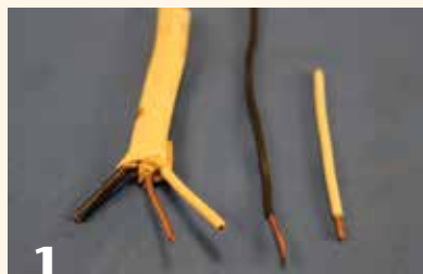
1 The copper core of 14/2-gauge electrical wire is a good choice of pin material.
