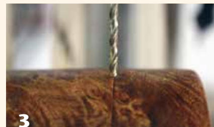
2 Tape the lid to the box securely before drilling. Use a shopmade V-block to hold the round box and then drill a pinhole centered on the box/lid juncture.
