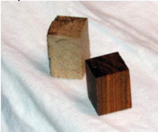
Select the blank of wood. I usually start with stock that is at least  $\frac{3}{4}$  inch square but larger or slightly smaller will work. Cut the wood to lengths anywhere from  $\frac{3}{4}$  to 3 inches. If your saw doesn't leave a beautiful finish, you should true the end on a sander. Drill the approximate center
