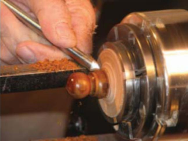
**Turning the wood to shape, in this case a neat knob.**
