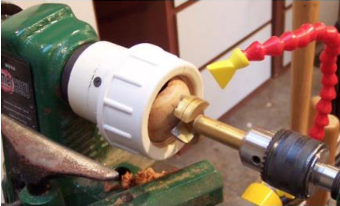
Picture 3: This set up shows the operation of drilling the first step at any given position. Note the mark on the drill which was made after the first hole was drilled in the ball.
