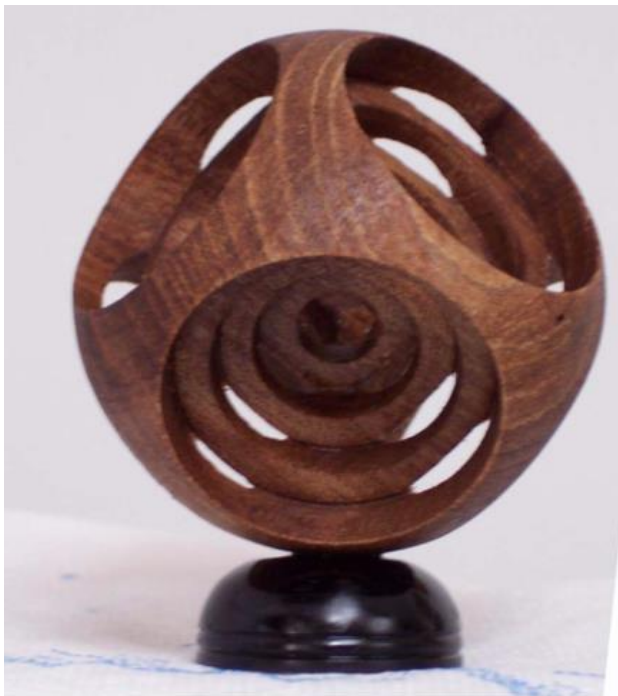
Picture 1: This was my first successful attempt to make this project. It is made from Elm and has an African Blackwood base. All holes were drilled with Forstner bits.
