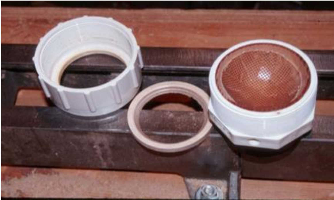
Picture 7. This photo shows the basic components of the ball chuck that I use. Left to right: screw on cap, plywood washer to fit between the sphere and the cap, male part of the PVC compression fitting is fitted with a hardwood block with a spherical recess. This one has sandpaper glued in to grip.
