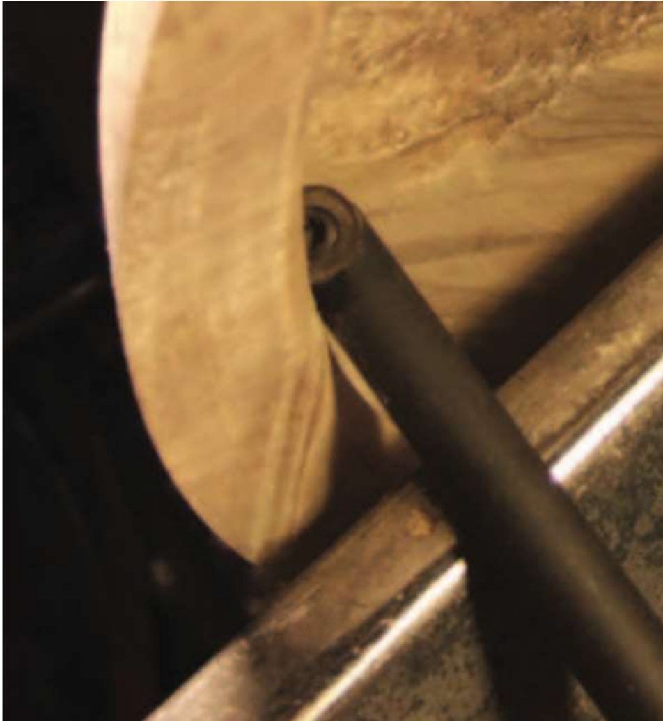
Figure 2. Undercutting the rim with the 3/8" Hunter Carbide Tool.
