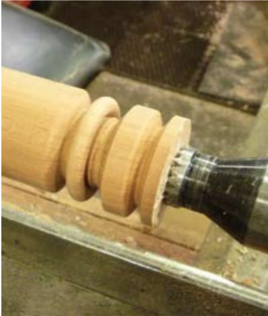
Figure 4. Here the ring is nearly cut loose. I finally cut the ring loose with the tool on the left side of the ring.
