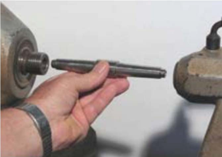
Figure 2. Using the Acruline System to check alignment.
