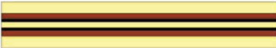
Now set up your saw for making cuts at the angle specified in your design. For this one, it's 30 degrees. Also set up a stop block so that all the strips will be cut at the same width. And, be sure the saw blade is 'dead on' vertical. The lamination board needs to be as long as needed for the strips plus some extra for safe handling during the sawing operation. After sawing, you now have this assembly of pieces:
